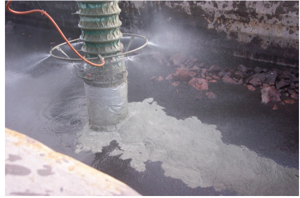
Pneumatic feed system with misting ring
