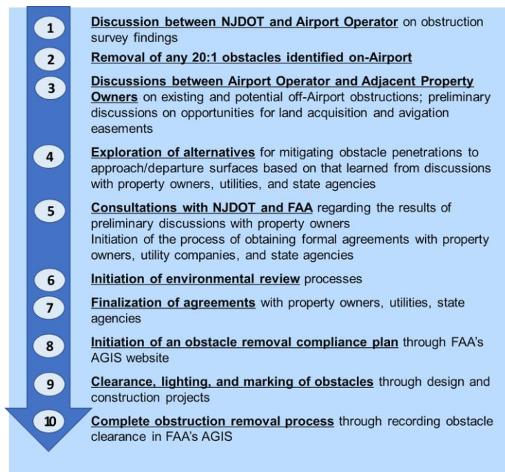
Figure 8-10 Obstruction Mitigation Process for New Jersey Airports
