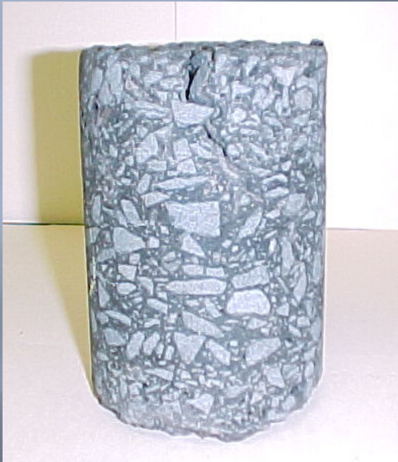
Top Down Cracking
