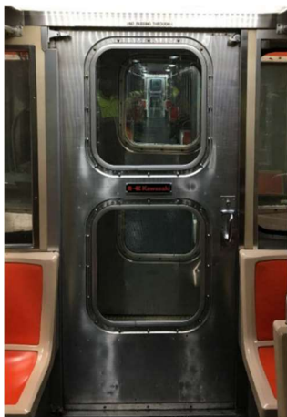
Figure 2-4: SEPTA door warning at time of accident, "NO PASSING THROUGH"
